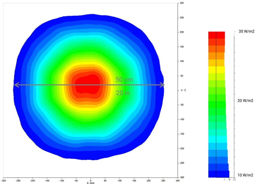
Distance to the surface 38 cm (15 in) | Conversion:  $3500 \mu\text{W}/\text{cm}^2 = 35 \text{ W}/\text{m}^2$
